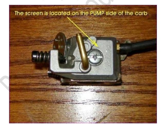
The **primary screen** is located on the **PUMP SIDE** of the carburetor. Remove the single screw located in the middle of the pump cover and carefully lift off the cover & rubber gasket, noting the position of the gasket. When
