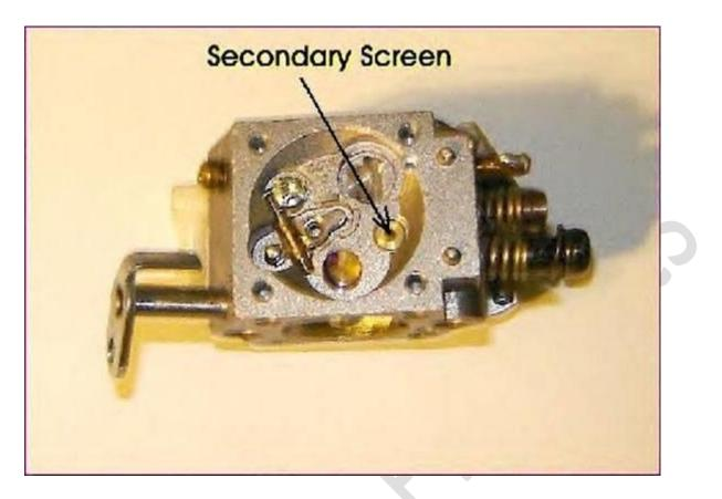
If one has a **Walbro** carburetor with a Secondary Screen, it is located on the **"float"** side of the **carb**, requiring the removal of 4 screws at the corners of the float diaphragm cover, and then careful removal of the float diaphragm. There is a brass insert as shown in the photo above and has a screen installed below the insert.
